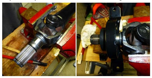
Next, realign the loose end of the drive shaft with marks that you made earlier and slide it up as far as you can. With a block of wood at the other end, hammer the driveshaft and bearing back into place.
