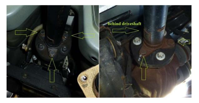
This would also be a good time to inspect the flex discs for cracks and damage, and replace them if needed (replacement of the flex discs requires additional tools). Mine were in good shape so I left them alone. Remove the nuts and washers but leave the bolts intact. Then brace the driveshaft while you remove the 13mm bolts that attach the bearing bracket to the underside of the car. (See below image)
