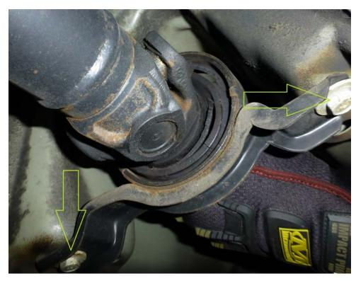
After removing the bolts, continue to brace the driveshaft and have the second person remove the loose bolts from the ends. Remove the driveshaft from the vehicle. With it out from under the car it is much easier to see the extent of the damage.
